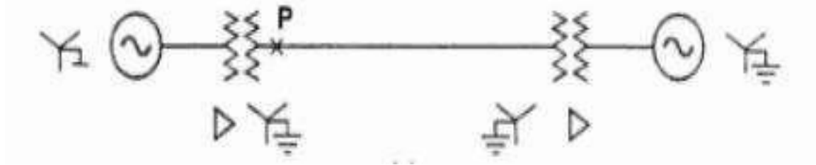
Figure 19 Single line diagram of a balanced 3-phase system
